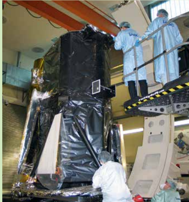
The eROSITA-instrument was specifically designed at MPE to scan the entire sky with its seven X-ray telescopes. Each contains 54 nested special mirrors. Its large field-of-view together with its high sensitivity for X-ray radiation promises the most accurate all-sky map of the X-ray background.
