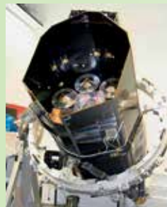
The eROSITA-instrument was specifically designed at MPE to scan the entire sky with its seven X-ray telescopes. Each contains 54 nested special mirrors. Its large field-of-view together with its high sensitivity for X-ray radiation promises the most accurate all-sky map of the X-ray background.
