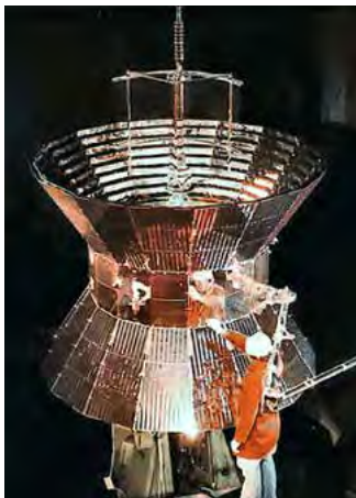
← The two Helios spacecraft launched in 1974 and 1976 were a very successful German-US collaboration to study interplanetary magnetic fields and particles.
