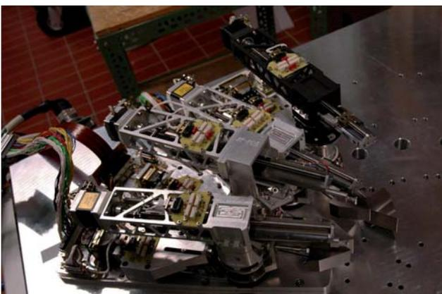
Fig. 2: Four KMOS arms during tests in the USM laboratories.
