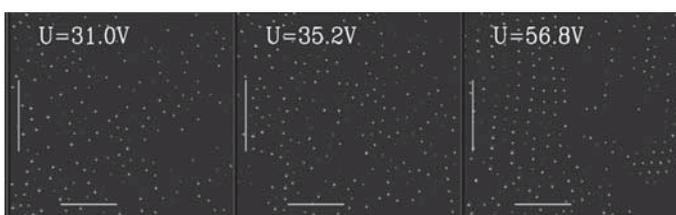
Fig. 2: First observation of the transition of an isotropic fluid into a string fluid in an electrorheological plasma. The control parameter is the voltage applied to the electrodes.
