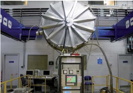
Fig. 1: The cryogenic part of KMOS on the Nasmyth flange simulator.
