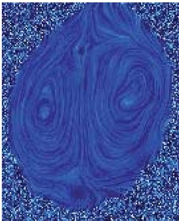
Fig. 3: Streamlines of the microparticles moving inside a droplet.
