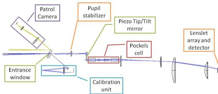
Figure 9 Optical design layout of the SH WFS.
