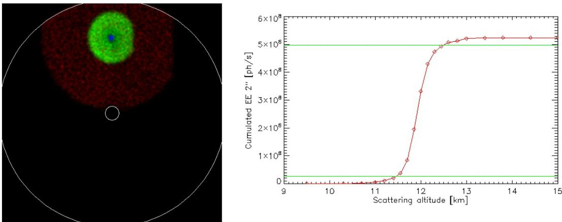
Figure 12 Left: Patrol camera images of light backscattered from different altitudes (red = 9.5km, green = 11km, blue = 12km). Intensities are not in scale. The 2 circles define the annular patrol camera FoV. Right: Flux in a 2x2 arcsec square around the peak. 90% of the intensity of peak comes from between 11.5 km and 12.5 km. Intensities are scaled to correspond to the nominal return flux (1800ph/ms/subaperture integrated from 11.85 to 12.15km)
