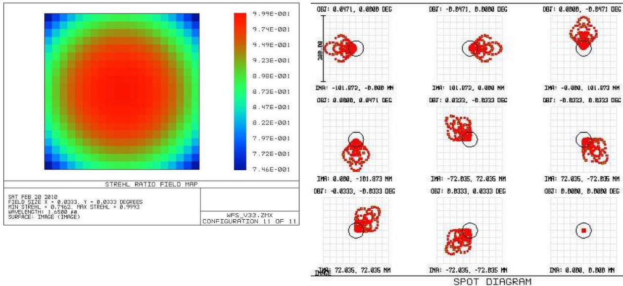
Figure 3 Optical performance of the pure LBT telescope. No dichroic is considered. Spot pattern and SR as a function of FoV position. Maximum distance is  $2\sqrt{2}$  arcmin to probe the square  $4\times 4$  arcminutes FoV of LUCIFER.
