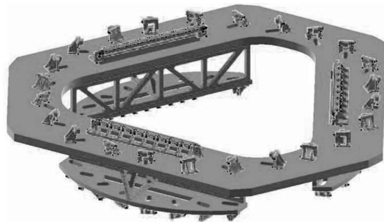
Fig. 3. Mechanical layout of the IFU module. Light passes through the optical bench from below and reflects off one of the individually mounted fore-optics mirrors. The light path returns to the second set of fore-optics which are located on a secondary optical bench mounted on standoffs from the main bench. The third fore-optics mirrors, the slicers, pupil mirrors arrays and slit mirror arrays are all mounted directly off the main optical bench.
