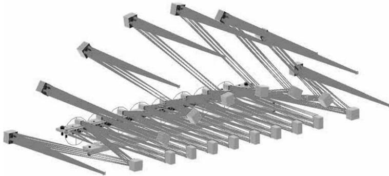
Fig. 2. Optical layout of the IFU optics in a single IFU sub-module. There are 4 different fore-optics designs in each sub-module of 8 IFUs but common slicer, pupil mirror array and slit mirror array designs. The optical design has also been optimised to put these common components in the same planes for easier mechanical mounting and production.
