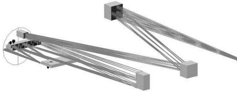
Fig. 1. Optical layout for a single pickoff field showing the three mirrors in the anamorphic fore-optics, the image slicer and the monolithic pupil mirror and slit mirror arrays.
