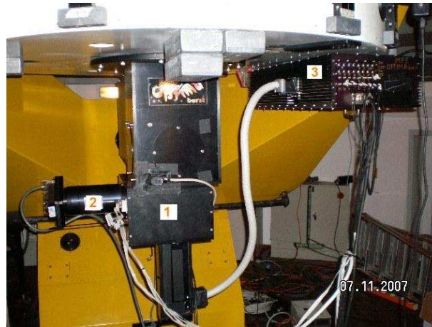
Figure 3.2. A photograph of OPTIMA-Burst mounted on the 1.3 m Cassegrain focus telescope of the Skinakas Observatory. The target acquisition optics (filters, target imaging and fiber pick-up) is located in box no. 1 and the CCD camera is mounted externally box no. 2. APD photon counters are located in box no. 3 connected to the telescope
