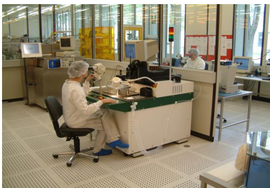
Fig. 2: The mounting area includes a water-guided laser dicer (back left) and an automatic bonder.
