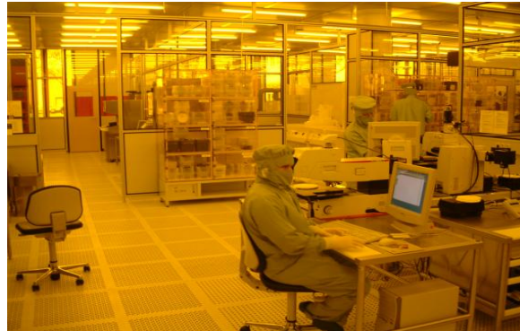
Fig 1: The part of the production area, shown here, contains an 8-tube furnace (back left), inspection (front) and wet etching equipment (back right).
