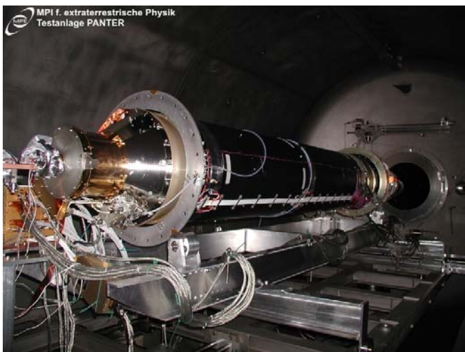
The Swift XRT pointing to the 1m aperture of PANTER's 130m long X-ray tube (right back).
