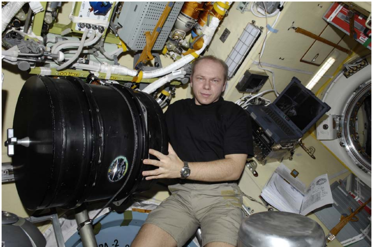
Figure 1: Cosmonaut Oleg Kotov with the PK-3 Plus laboratory in MIM-2, the new Russian docking and research module, after installation of the experiment apparatus (front, in the black barrel) and the control computer (behind the cosmonaut). (Credit: Image courtesy of RKK-Energia).
