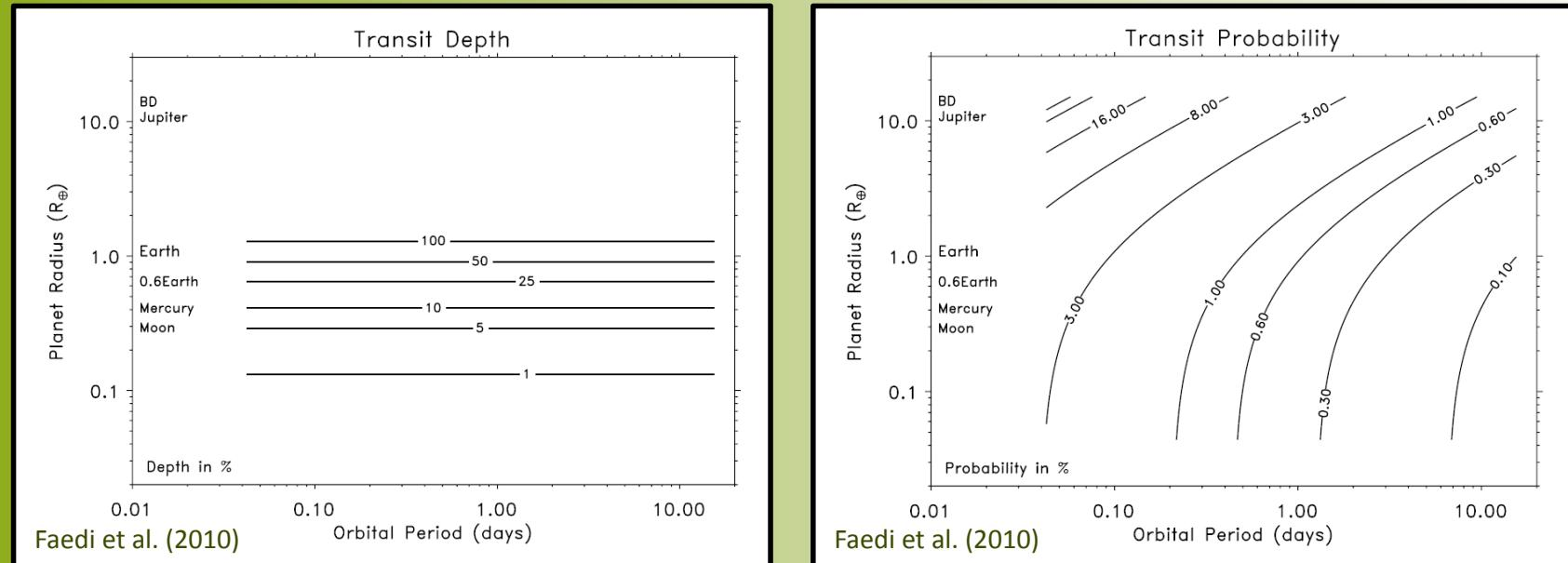
$$\delta_{tr} = \frac{\Delta F}{F} = \begin{cases} R_p^2/R_*^2 & \text{for } R_p \leq R_* \\ 1 & \text{for } R_p > R_* \end{cases}$$
