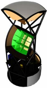
Fig. 1 [Left] The “reference design” of EXIST, with three Tungsten coded-mask imaging telescopes ( 2.7 \text{ m}^2 of CZT per telescope). Fig. 2. [Right] Sensitivity estimate ( 5\sigma , 1yr survey) based on an exposure time of 10^7 \text{ s} , allowing for 20% source duty cycle. Estimates of the continuum sensitivity assume \Delta E/E = 1 , and for lines \Delta E/E = 0.01 . The actual FWHM energy resolution below 150 keV will be less than 1 keV. Above 150 keV, Compton events will reduce the resolution.
