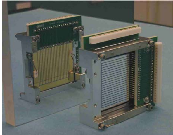
Figure 4 Photo of double-sided Si(Li) strip detector fabricated at LBNL. The boron-contact side is seen in the mirror.
