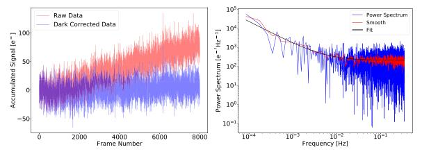
**Figure 2.** Left panel: readout noise obtained from the ramp data after dark and pixel reference correction for an inner pixel of the NISP array. Right panel: we show the time power spectrum for the left panel readout noise (blue), the smoothed power spectrum (red), and the best-fit  $(1/f)^{\alpha}$ -like model (black).
