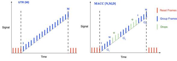
Figure 1. From left to right, we present a schematic view of the Up the Ramp (UTR), and Multiple Accumulative (MACC) read modes, respectively. The reset, acquired, and dropped frames are shown in red, blue, and green.
