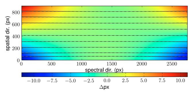
**Fig. 2.** The anamorphic distortion of the LRS as mapped by tracing the peaks of the stellar spectra. The traces of nine stellar spectra are shown as full black lines and are compared to the corresponding straight lines (dashed). The interpolated differences (in pixel) between the stellar traces and the cartesian grid as a function of the position on the chip are shown coded by color.
