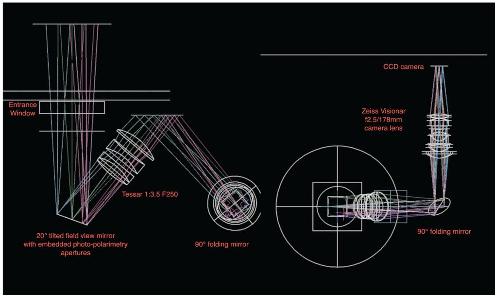
Fig. 2b: Field viewing optics (ZEMAX ray tracing) to provide an image of the environment around the photon counting apertures in the slanted mirror.
