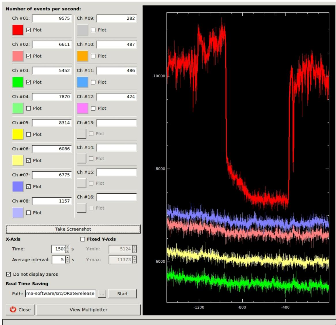
Fig. 4: Realtime display of rates for an eclipse of HU Aqr with 1 second resolution. Four channels of sky background intensity are also displayed (data taken at Skinakas observatory 2012)
