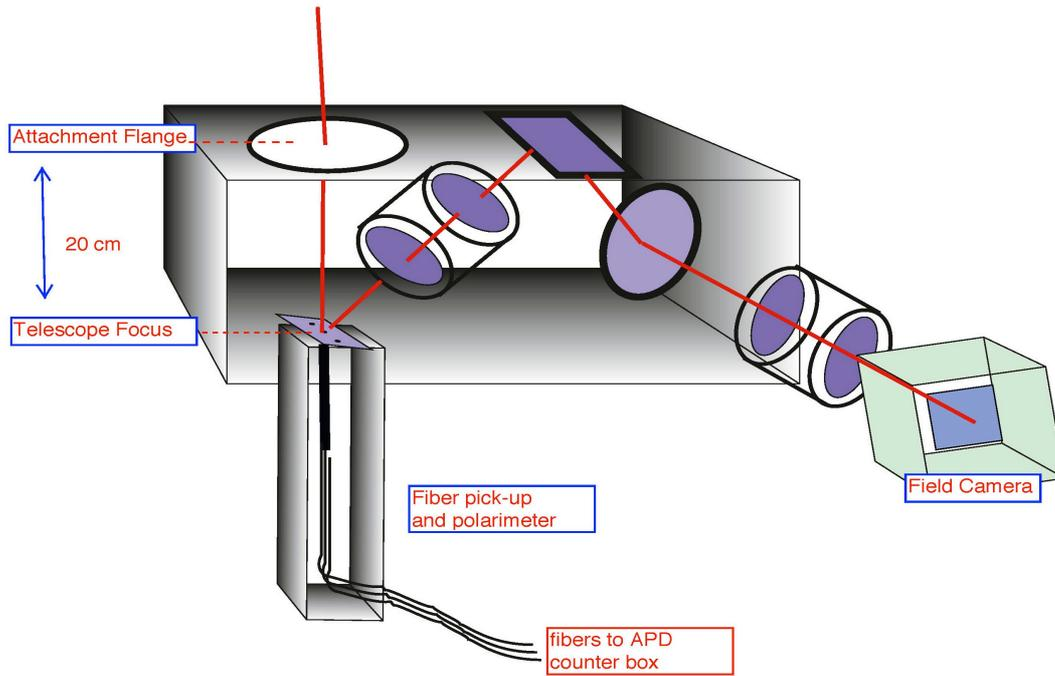
Fig 2a: Schematic of OPTIMA focal plane assembly (FPA)
