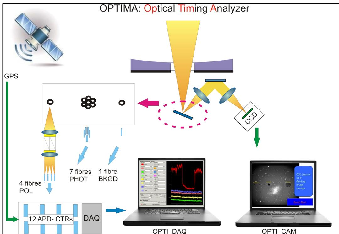
OPTIMA provides two principal modes of measurement, which can be selected by positioning a target on specific apertures embedded in the slanted mirror:
