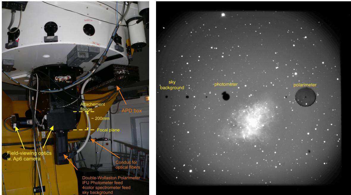
Fig. 3: (left) OPTIMA mounted on the Cassegrain focus of the 1.3m telescope on Mt. Skinakas, Crete (Greece). (right) Image of the Crab nebula in the field-viewing camera (SKO 1.3m, 2012). Apertures (fibre pick-ups) for the photon-counting modes are indicated.
