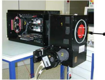
**Fig. 2.** Photograph of pre-2006 OPTIMA with open APD box of photon counters (3). The target acquisition optics (filters, target imaging and fiber pick-up) is located in box (1) and the CCD camera is mounted externally (2).
