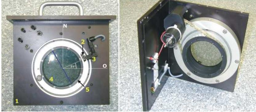
**Fig. 7.** Photograph of the OPTIMA rotating polarization filter. Left (seen from telescope side): 2: permanent magnet on rotating filter; the polarization direction of the filter (4) is perpendicular to the radius vector to the magnet. 3: Hall sensor on base plate. The filter rotates from north to east. Right: motor and belt. Typical rotation rates are 3-4 Hz.
