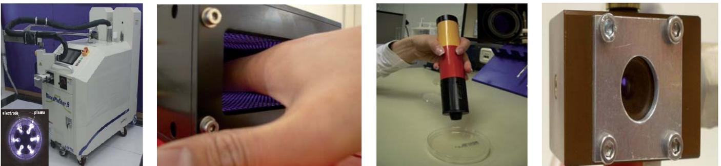
Fig. 1: Development of plasma devices using different plasma generating technologies. From left to right: The MicroPlaSter (torch type), HandPlaSter, PersonalPlaSter (BCD type) and VenturiPlaSter.
