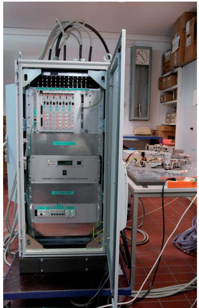
Fig.3: The cabinet, which is controlling one sector of KMOS.
