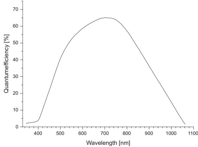
Figure 2. Quantum efficiency of the APD single photon counting modules from Perkin Elmer Inc.
