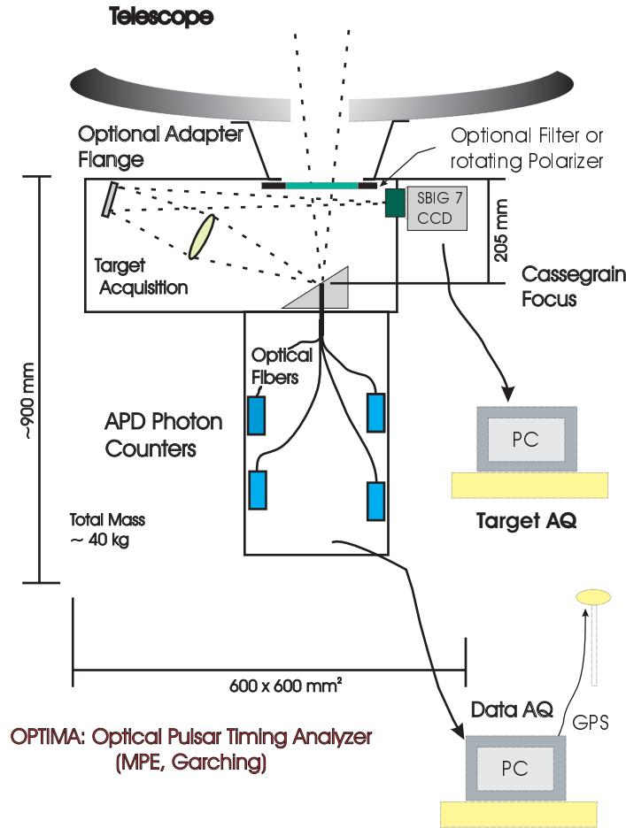
Figure 1. Schematic layout of OPTIMA
