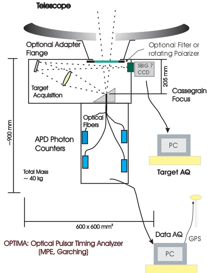
Figure 1. Schematic layout of OPTIMA
