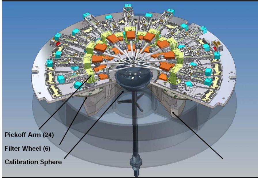
**Fig. 2.** An internal view of the KMOS cryostat showing the pickoff arms and the calibration unit fed through from the rear of the cryostat.
