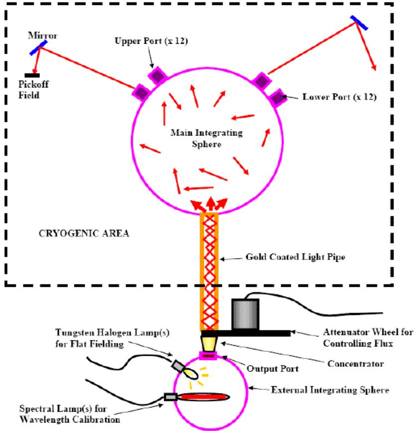
**Fig. 3.** This schematic of the calibration unit shows key features of the operation and design. Lamps are fed into the cryostat from an external integrating sphere. The light is reflected from mirrors mounted around the field lens into arms located at the calibration position.
