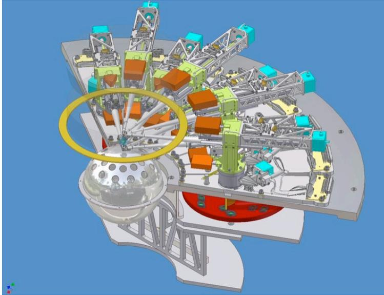
**Fig. 2.** One of the three integrated pickoff and IFU sub-modules showing the three mounting plates for the pickoff arms, the filter wheels and the IFU optics. Each sub-module is attached to the main cryogenic optical bench within the cryostat. At the centre of the unit is shown the integrating sphere of the calibration unit and the ring mirror which reflects light from the calibration sources in to the pickoff arms.
