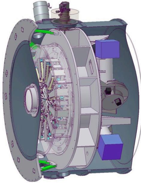
**Fig. 1.** Cutaway view of the main KMOS cryostat showing the entrance window and the pickoff arm module at the front, the IFU module in the middle and the spectrograph module at the rear. The cryostat will be an aluminium/stainless steel hybrid to reduce weight.
