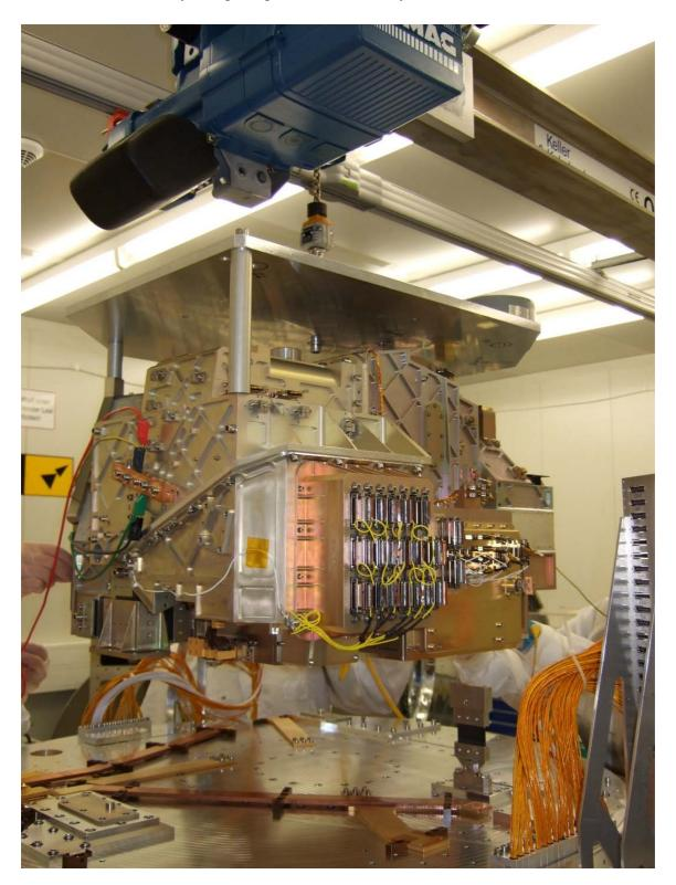
Fig. 2: Mounting of the PACS FPU to the test cryostat (today).
