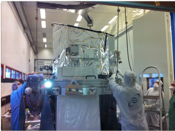
Getting ready to lift eROSITA into its clean container at MPE (left). Eventually, eROSITA is laid into its protective enclosure (right), ready to leave MPE and be shipped to IABG for the tests campaign.
