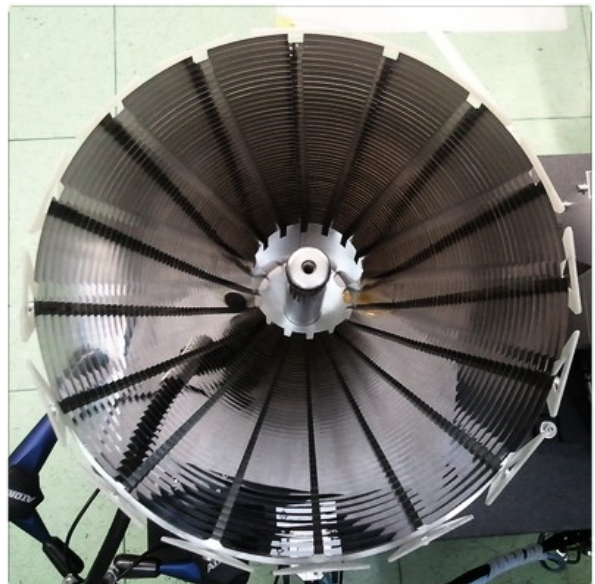
The first Flight Module X-ray Baffle in the MPE workshop at the end of October 2012.
