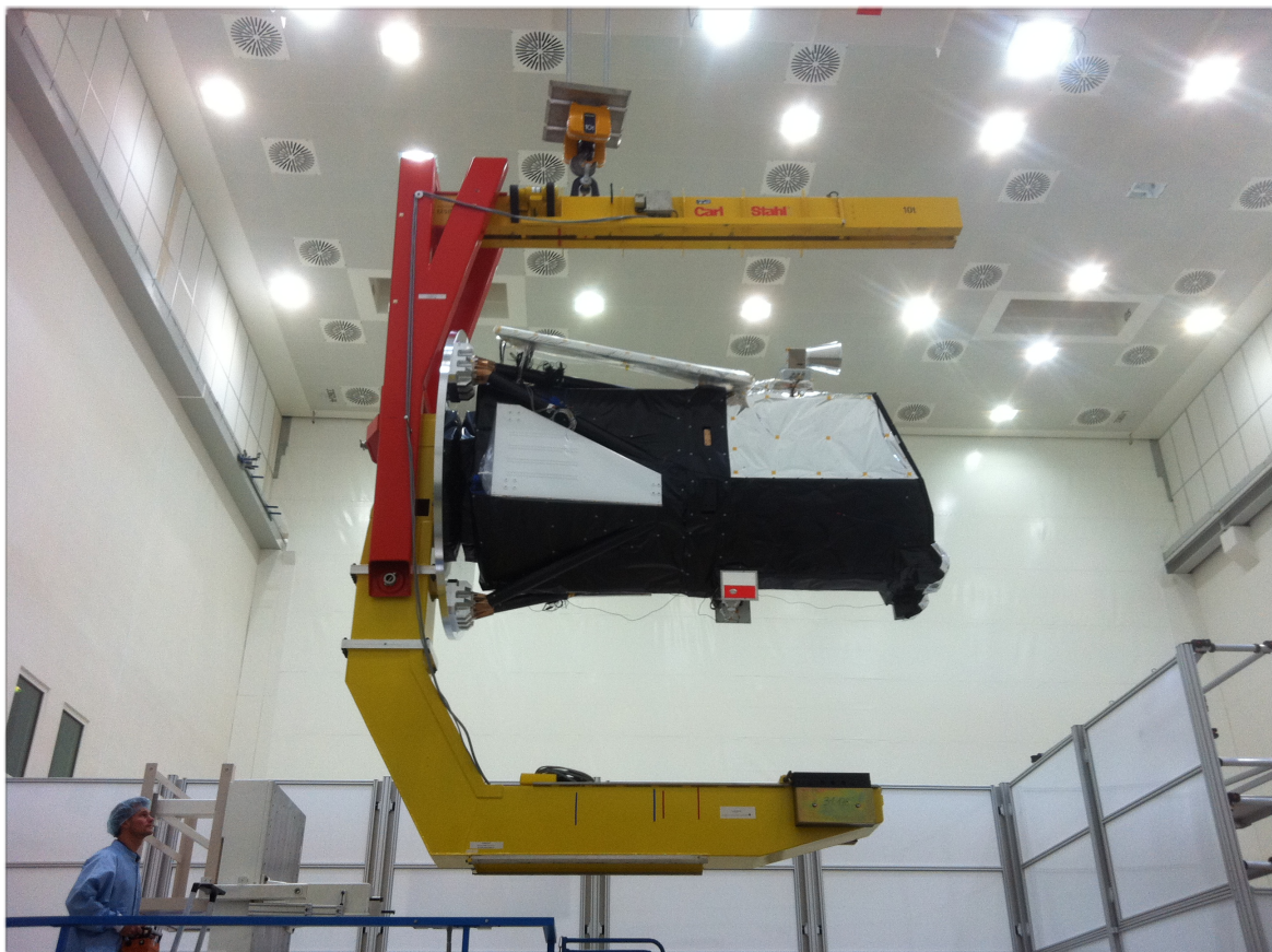
eROSITA at the space testing facility IABG during mass measurement.
