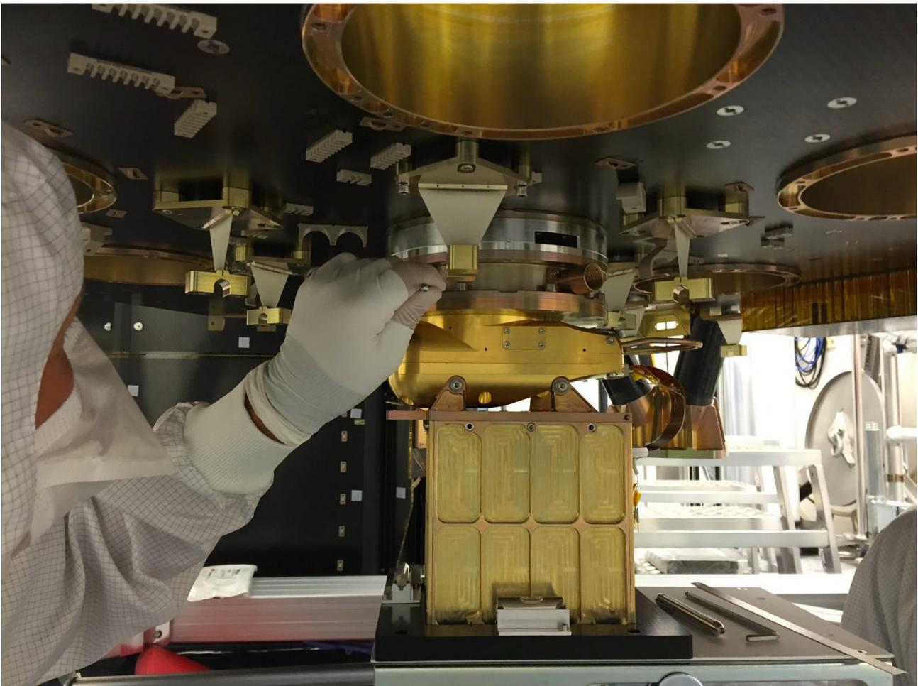
*The integration of the eROSITA Mirror and Camera Assemblies (shown here) requires an extreme accuracy: the individual focal length (1600mm) of each pair has to be matched within 50 $\mu$ m. The metrology system has been developed at MPE.*
