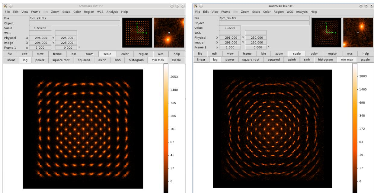
*PSF mapping at two different energies: Al-K $\alpha$  (left) and Cu-K $\alpha$  (right). The data were collected at PANTER during the test and calibration campaign of the Flight model mirror assembly FM2.*
