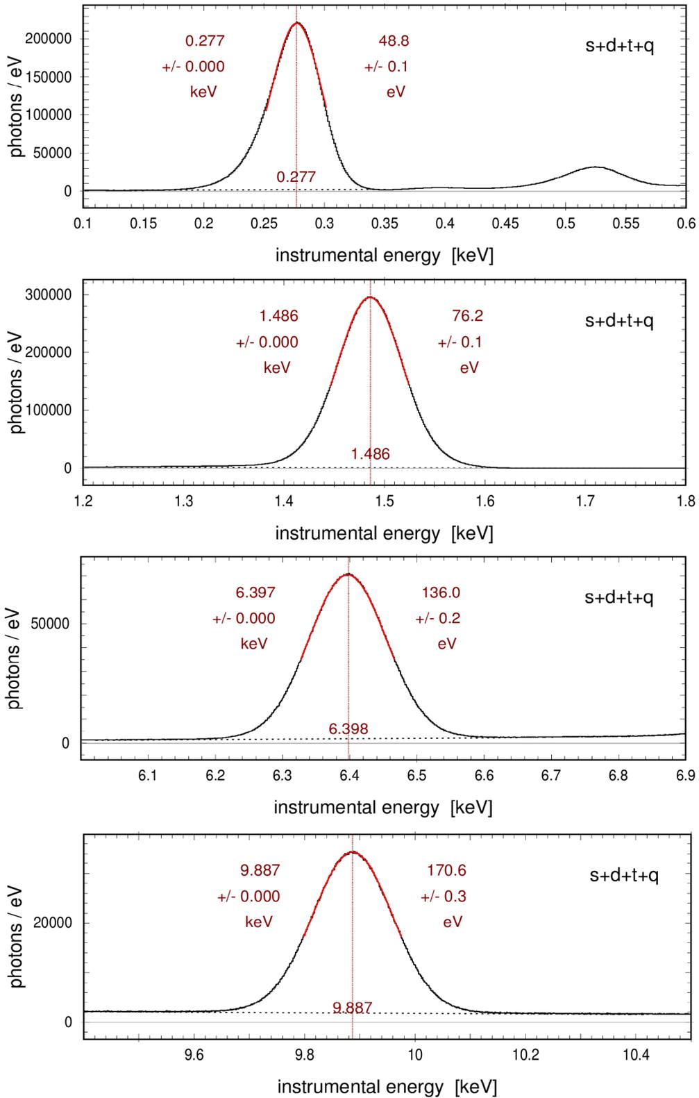
*FM1 camera energy resolution tests. From top to bottom, the four panels show the response to monochromatic illumination at the energies of C-K $\alpha$ , Al-K $\alpha$ , Fe-K $\alpha$  and Ge-K $\alpha$ , respectively. 's+d+t+q' means sum of singles, doubles, triples, and quadruples, i.e. all events are used for the energy reconstruction.*
