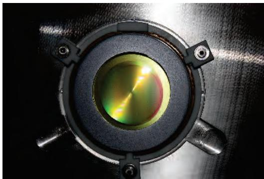
**Fig. 1:** Large area ZP ( $20 \text{ cm}^2$ ) mounted in the PANTER X-ray test facility.
