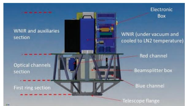
**Figure 2: Instrument overview:** Shown are the sections with the different elements.
