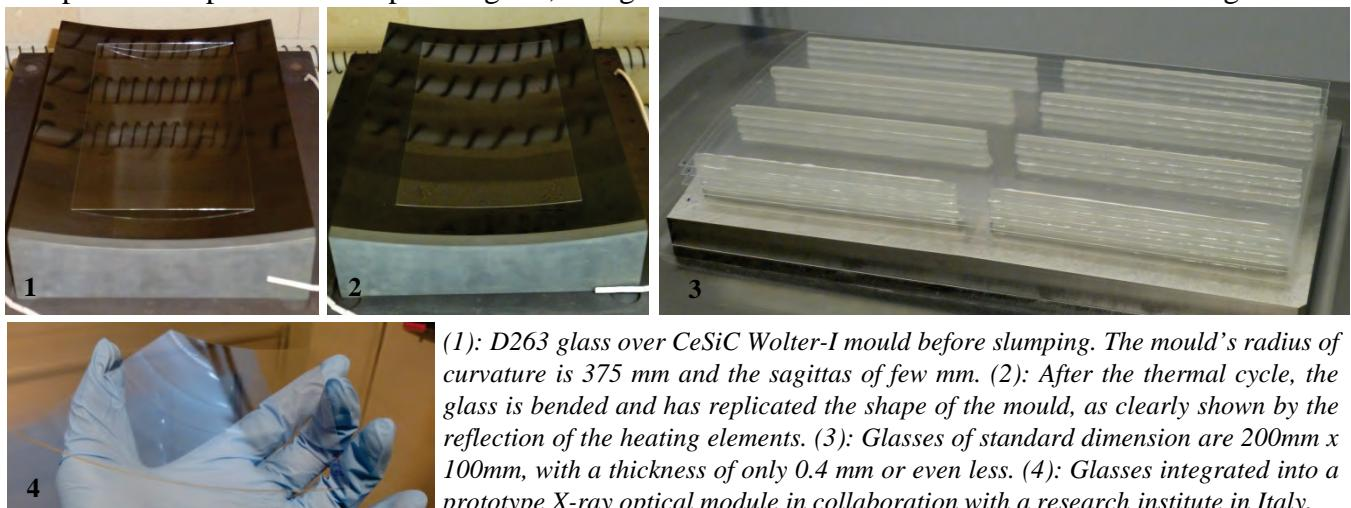
(1): D263 glass over CeSiC Wolter-I mould before slumping. The mould’s radius of curvature is 375 mm and the sagittas of few mm. (2): After the thermal cycle, the glass is bended and has replicated the shape of the mould, as clearly shown by the reflection of the heating elements. (3): Glasses of standard dimension are 200mm x 100mm, with a thickness of only 0.4 mm or even less. (4): Glasses integrated into a prototype X-ray optical module in collaboration with a research institute in Italy.
