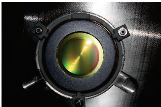
**Fig. 1:** Large area ZP (20 cm<sup>2</sup>) mounted in the PANTER X-ray test facility.
