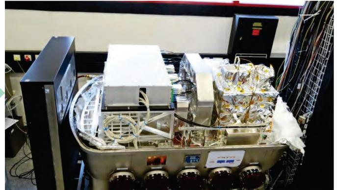
A LN<sub>2</sub> cryostat provides the operation temperature and stability for the beam combiner sub-units.
