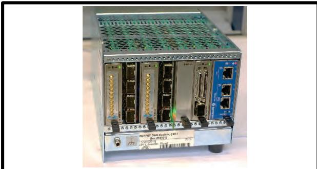
**Fig. 1:**  $\mu$ TCA data acquisition System (Rack)
