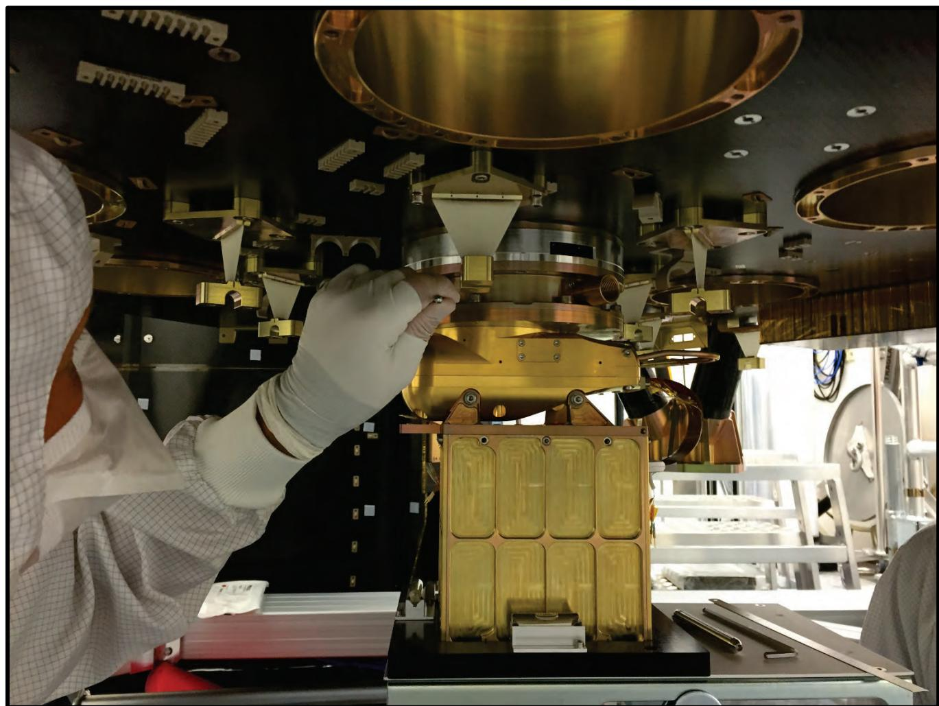
The integration of Mirror Modules and Camera Assemblies (shown here) requires an extreme accuracy: The individual focal length (1600mm) of each pair has to be matched within 50 $\mu$ m. The metrology has been developed at MPE.
