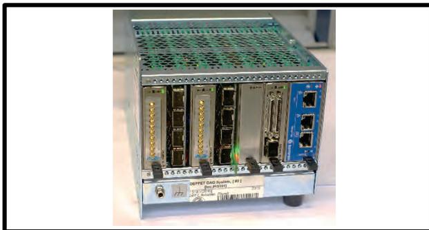
Fig. 1:  $\mu$ TCA data acquisition System (Rack)
