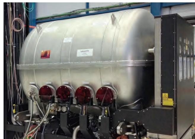
The GRAVITY cryostat in the integration hall at Paranal shortly after arrival. The instrument is cooled with liquid N<sub>2</sub> and sealed in a vacuum vessel. Isolated from ambient the instrument is extremely stable.
