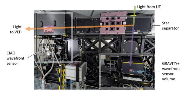
Figure 10: View of the coudé room below the UTs. The light from the sky and from the laser guide star enters the star separator (STS) module from top. The visible wavelengths (yellow) are transmitted toward the coudé focus behind the STS itself to feed the wavefront sensor (WFS). GRAVITY+ will upgrade the current WFS with a new state of the art WFS based on the ERIS design and will support both natural and laser guide stars.
