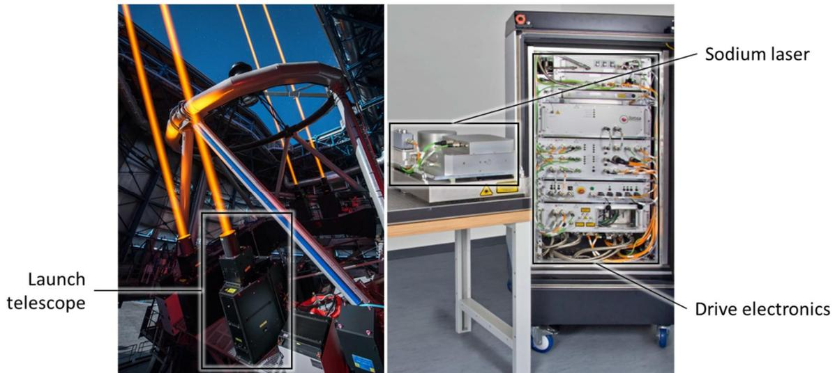
Figure 11: GRAVITY+ will equip UT1,2,3 with a laser guide star. The baseline is a replica of the AOF LGS, or an adaption of the upcoming ELT LGS. Left: AOF launch telescope (ESO/G. Hüdepohl). Right: SodiumStar (Toptica Projects).
