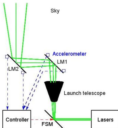
Figure 2. Set up, of the vibration compensation at the telescope.
