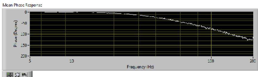
Figure 6. Frequency dependence of the phase shift of the PI mirror.
