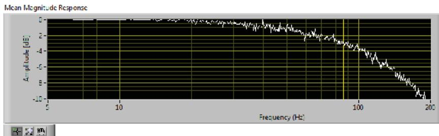
Figure 5. Frequency dependence of the amplitude response of the PI-mirror.
