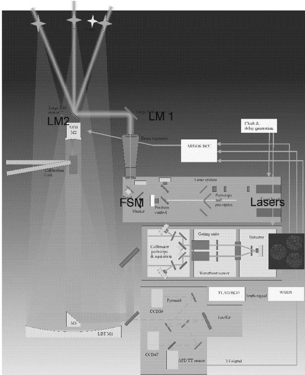
Figure 1. Sketch of the ARGOS system at the LBT. (Thanks to S.Rabien). The important components of the laser launch path are the fast steering mirror (FSM) and the two folding mirrors (LM1, LM2).
