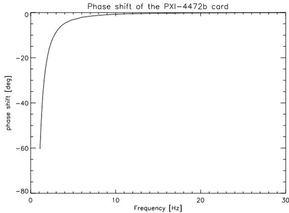
Figure 4. Frequency dependence of the phase shift of the PXI-4472b card
