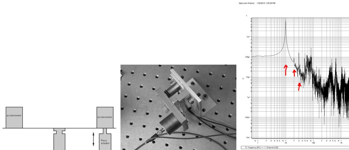
Figure 7. Left: Principle of the mechanical set-up for the vibrating mirror. Center: Picture of the mirror with one accelerometer attached. Right: Power spectrum (acceleration) of vibrating mirror. The scale is logarithmic. The excitation was at 10 Hz the next two overtones and the high frequency noise are clearly visible.
