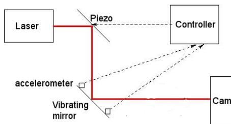
Figure 3. Laboratory set up: The light from the laser is deflected off the FSM, then off the vibrating mirror which introduces the 'telescope vibrations' into the beam, and finally monitored on a CCD .
