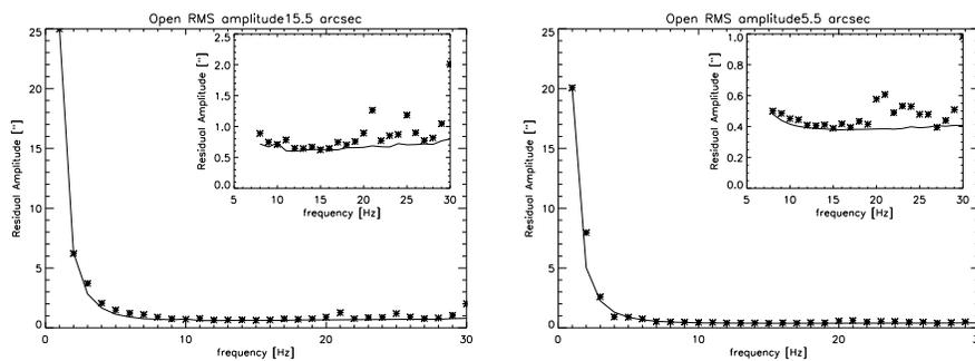
Figure 8. Left: Comparison of the performance of the system for large amplitudes (15''4 RMS). Right: The same for amplitudes as expected at the telescope (5''5 RMS). The inlay shows the results for frequencies of 7Hz and higher.
