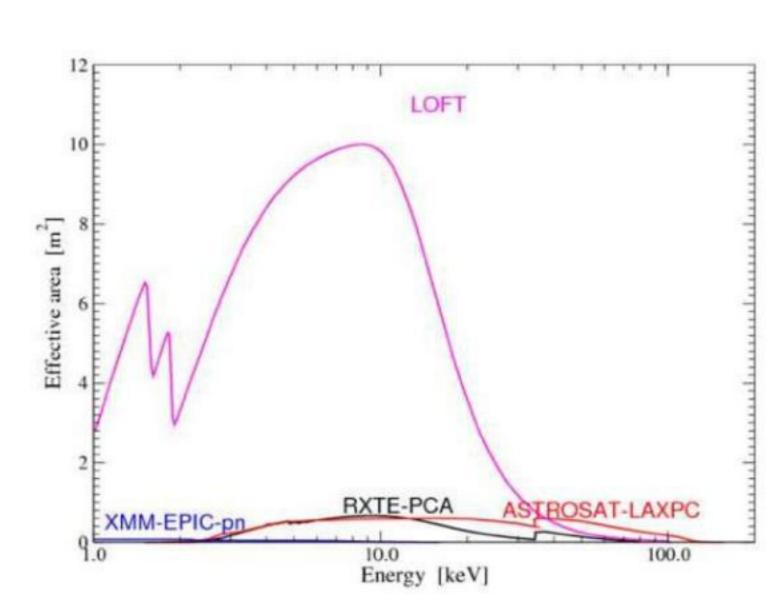
Left panel: Sketch of the LOFT satellite. The 6 deployable panels of the LAD, the WFM and the solar array are indicated. Right panel: effective area of the LOFT/LAD as a function of energy
