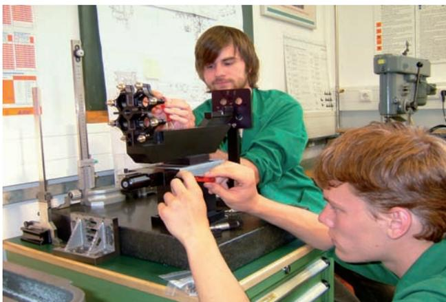
Fig. 2: Mounting an optical experimental-setup to test the PRIMA instrument by 3rd year apprentices.
