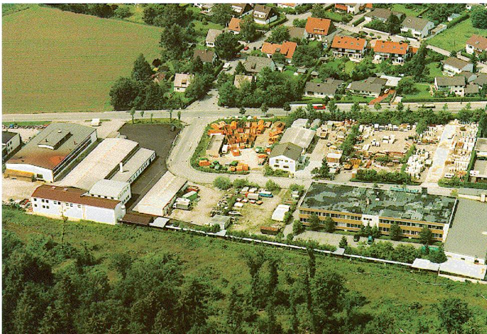
Fig. 2: An aerial photograph of the MPE Panter X-ray test facility in Neuried. The X-ray source and the telescope chamber are separated by a 130m vacuum pipe system.
