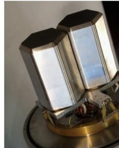
**Figure 3.3:** The two SPITS Ge detectors without the Al vacuum cap. Photograph courtesy of Eurisys Mésures.
