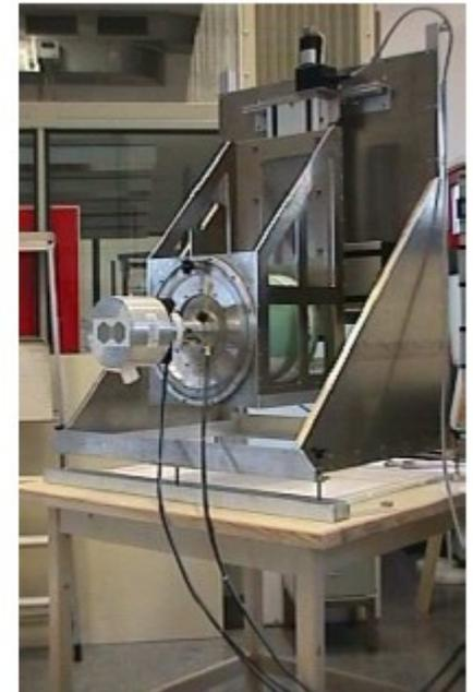
**Figure 3.4:** The SPITS Ge detectors with nitrogen dewar, mounted on the XY-table.
