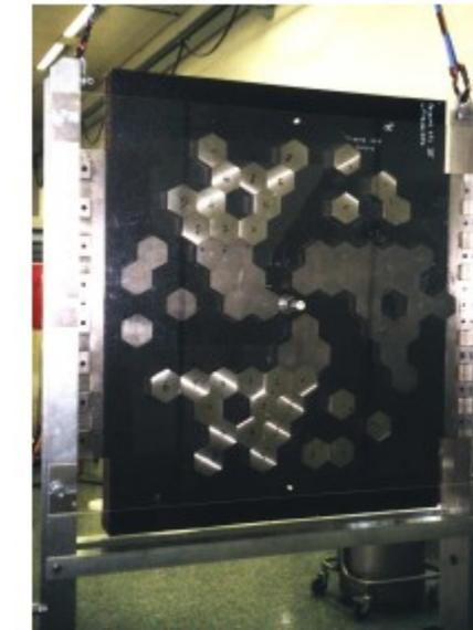
**Figure 3.2:** The fully assembled SPITS mask with plexiglass sheet and support.
