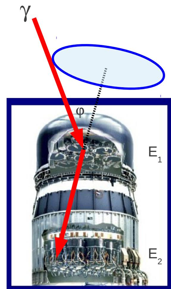
Double Compton scattering: scatter-angle is function of measured energy loss  $E_1$  and  $E_2$ .
