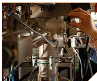
Isotope composition in meteorites can be analysed at the nanoscale using a type of mass spectrometer called a nanoSIMS
